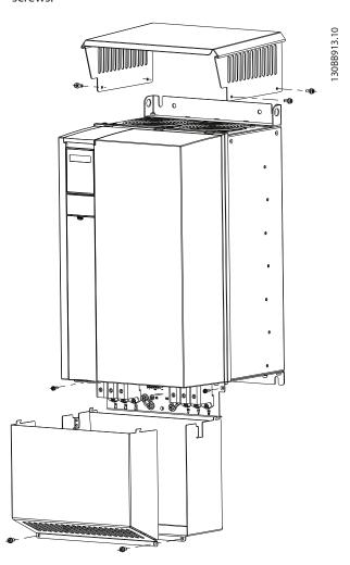
**Step 2**Fit bottom cover onto frequency converter and tighten an M4 screw.
