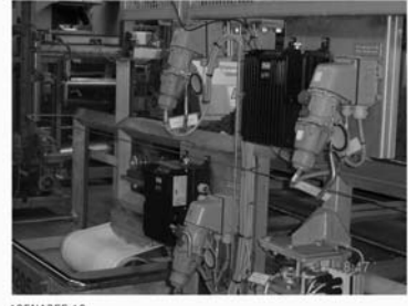
Illustration 1.17: Efficient space utilisation in the food industry with decentralised motor controls from Danfoss
