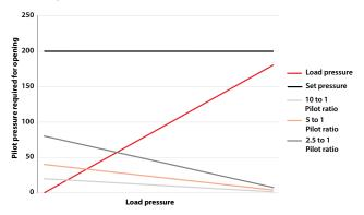
Instability results from rapid changes in the load pressure. In the chart above, you can see how a lower pilot ratio valve (2.5 to 1) has greater sensitivity to changes in the load pressure. In other words, if the load pressure suddenly increases, the operator will have to apply additional pilot pressure. A higher pilot ratio valve, with a flatter response, is more likely to open quickly when a sudden increase in load pressure occurs.
