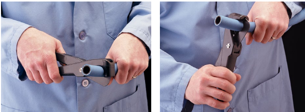
The rotating/rocking technique produces fast easy cuts.
