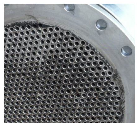
New/cleaned turbular heat exchanger.
