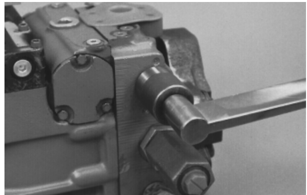
Fig. 2 - Install and Torque Cartridge (Typical)
