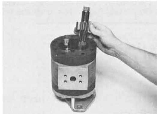
Fig. 51 -- Install Drive Gear
