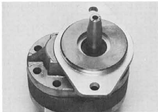
Fig. 30 -- Install Flange Assembly
