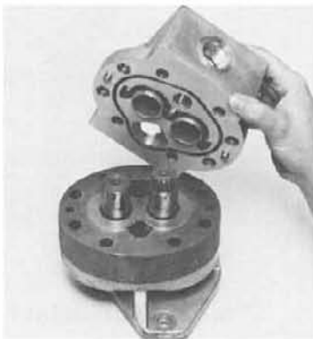
Fig. 43 -- Remove Cover from Single Pump
