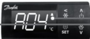
Temperature and alarm codes alternate flashes until the alarm is resolved. The alarm bell is shown.
