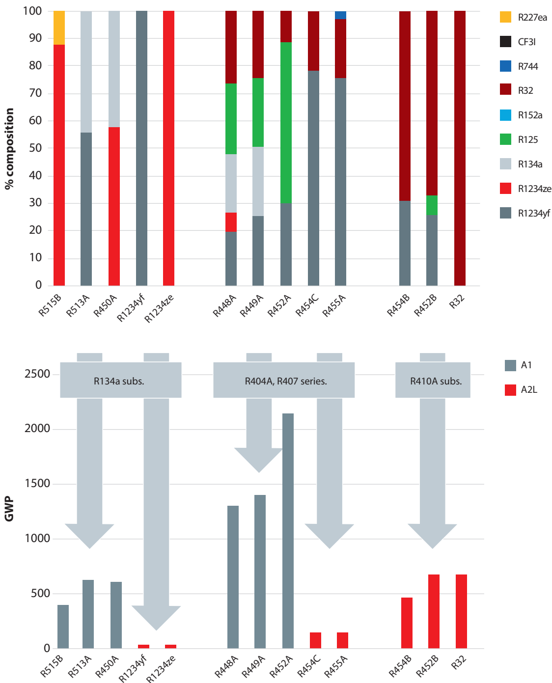
Figures 12a and 12b: The main replacement options and their composition and GWP levels.
