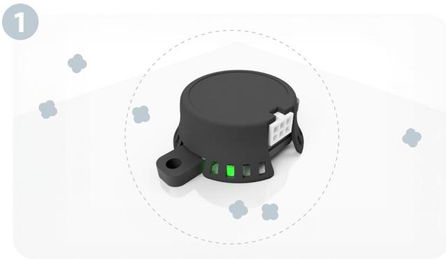
The TC sensor uses the thermal transfer properties of gases as a measurement tool for the presence of gas. The thermal conductivity of gases is inversely proportional to molecular weight. Therefore, thermal conductivity decreases with increasing molecular weight.
