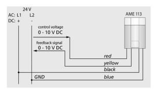
The actuator is controlled via a 0-10 V control unit or a building management system.
