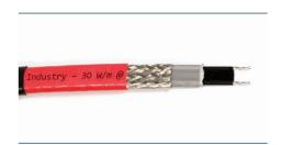
DEVIpipeguard™ Industry is a self-limiting heating cable that is mainly used for frost protection of pipes and for temperature maintenance in applications up to 120 °C powered or 190 °C unpowered cable. The cable allows steam cleaning in pipes. The heating element, the insulation and the outer jacket of
