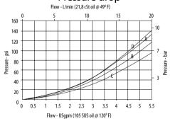
**A-**Port 3 to 2 (actuated) • **B-**Port 3 to 4 **C-**Port 2 to 1 • **D-**Port 4 to 1 (actuated)
