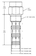
Installation torque A-47-54 Nm [35-40 ft. lbs] S-68-75 Nm [50-55 ft. lbs]
