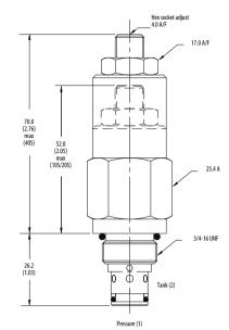
Installation torque A - 47-54 Nm [35-40 ft. lbs] S - 68-75 Nm [50-55 ft. lbs]
