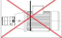
When lifting the pump unit, one sling must be attached to the electric motor and one sling around the pump.
