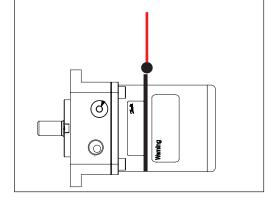
When the pump is mounted together with an electric motor, the pump unit always weigh more than 20 kilos and must be handled by using slings around the pump unit.
