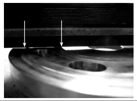
A good way to identify a worn valve plate is to hold a straight knife edge over the valve plate. When holding it up to the light, it will be possible to see any space between the knife edge and the valve plate. See picture 3.
