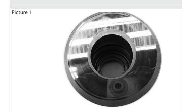
If the swash plate is polished 360°, it is an indication of insufficient filtration.
