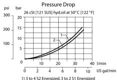
1) 3 to 4 S2 Energized, 3 to 2 S1 Energized 2) 2 to 1 S2 Energized, 4 to 1 S1 Energized
