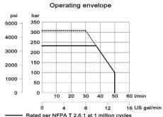
Rated per NFPA T 2.6.1 at 1 million cycles ------ Rated per NFPA T 2.6.1 at reduced operational life
