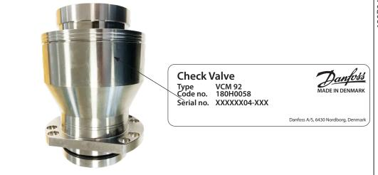
The non-return valve is designed for use in Seawater Reverse Osmosis (SWRO) membrane systems. In case the high-pressure pump stops momentarily, the volume of water in the membrane vessel may work as an accumulator and will send flow backwards.
