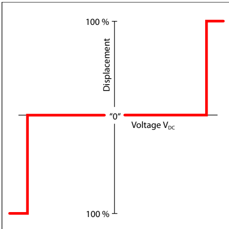
Pump displacement vs. electrical signal
