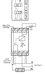
The screen of the heating cable must be connected to the earth conductor of the power supply cable by using a separate connector.
