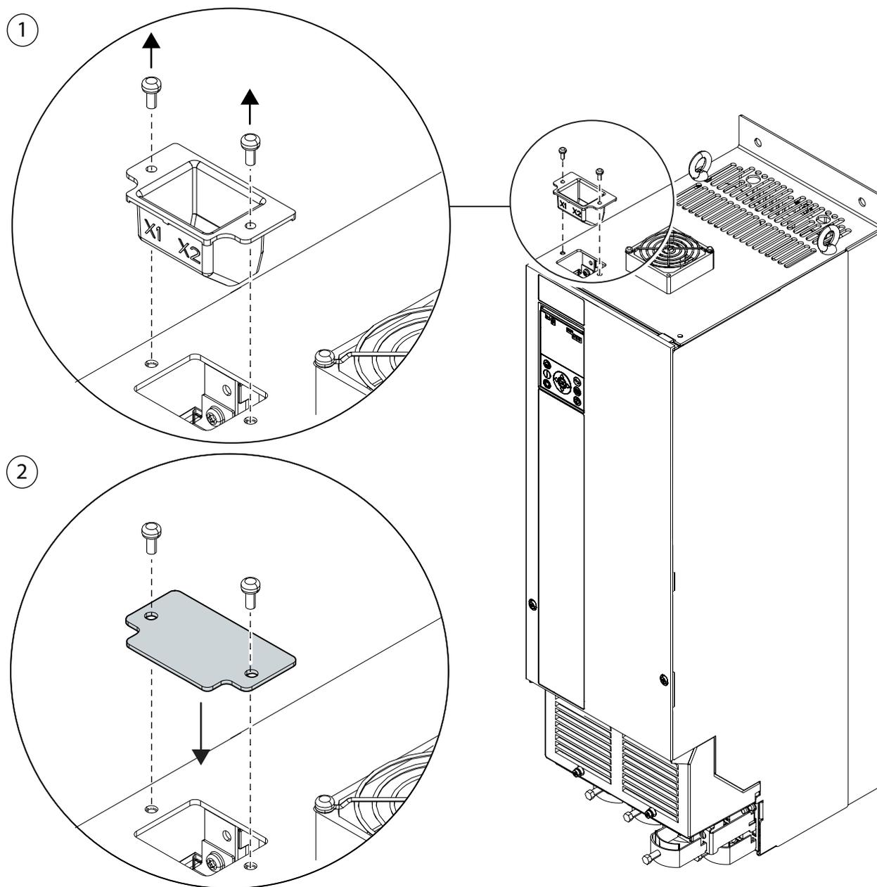
**Figure 1: Top Cover Plate Installation**
