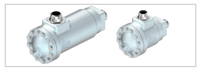
We are pleased to announce that Danfoss is launching DCR semi-hermetic filter driers for the  $CO_2$  applications. These new driers are designed for 90 bar working pressure and -55 to 100°C operating temperature, suitable for sub-critical and trans-critical refrigeration systems.
