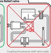
Coupling the pressure relief valve outlet directly to the pump inlet may damage the pump
