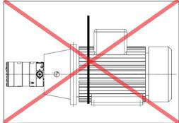
When lifting the pump unit, one sling must be attached to the electric motor and one sling around the pump.
