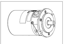
Pumps which have a weight above 20 kilos (see appendix 1, Data sheet) must be handled by using lifting eyes and slings.
