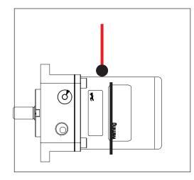
When the pump is mounted together with an electric motor, the pump unit always weigh more than 20 kilos and must be handled by using slings around the pump unit.
