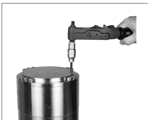
31. Tighten 10 screws to 30Nm.
