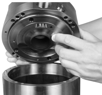
5. Mount port flange on housing. Use pin as guide.
