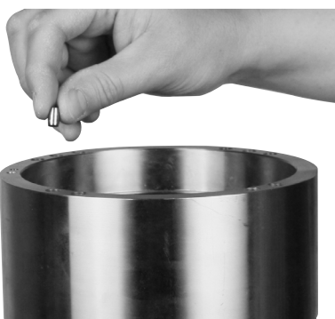
9. Mount 1 guide pin inside the housing on the back side of the port plate.
