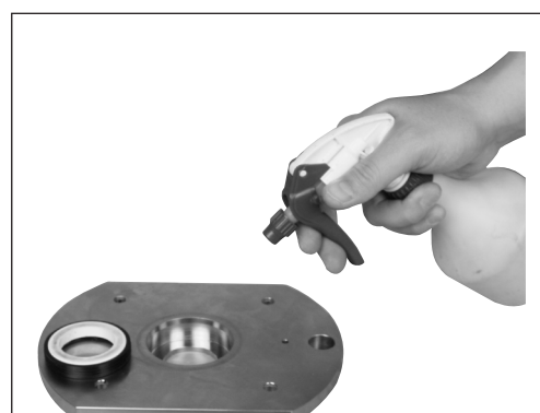
34. Spray shaft sealing with water before mounting.
