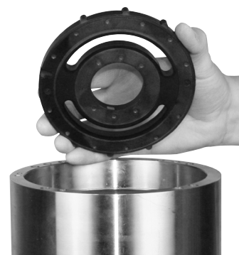
10. Mount port plate. Be aware of orientation/ guide pin.
