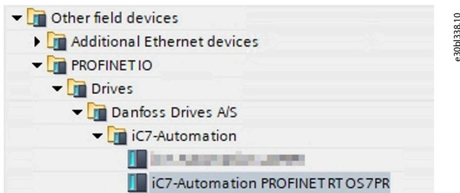
Figure 6: Example (iC7 Automation Series): Instance of Current GSD File
