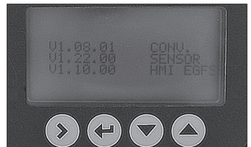
Display after power on.
