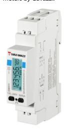
The 1-phase energy meter EM 511 can be installed in any low-voltage switchboard with rated current up to 45A to monitor the energy consumption, the main electrical variables and the harmonic distortion.
