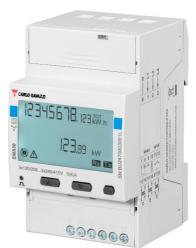
The 3-phase energy meter EM 530 can be installed in any low-voltage switchboard, to monitor the energy consumption, the main electrical variables and the harmonic distortion. Compatible with any current transformer with 5 A secondary current, it can be installed in systems with rated current up to 10 kA, even in retrofit applications if used with openable transformers.
