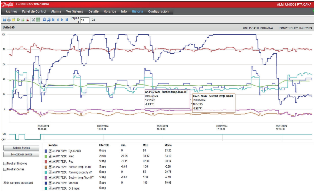
The graph above demonstrates the 5-degree Kelvin difference (average value) between the saturated temperature in the MT compressors' suction line and the evaporator's exit temperature. The screenshot from Danfoss's System Manager AK-SM 850 captures the Unidos Punta Cana store's liquid ejector performance over a typical two-hour period.
