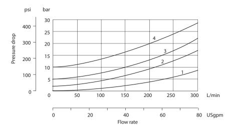
Port B to A, piloted open ..... Curve 1
