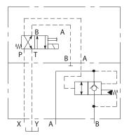
Solenoid controlled pilot operated check valve with externally drained pilot piston, PCG5V-\*\*(D)- 1, 11 and 20 series
