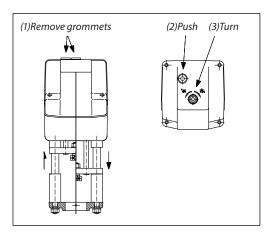
The manual override is applied by rotating the 8 mm Allen key (not supplied) to the required position. Observe the direction of the rotation symbol.
