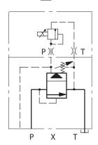
KCG-6/8 with manual and electrical pilots drained to side drain port ◆: Model code 7 = 1
