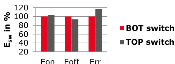
Figure 12: Differences in switching energy dissipations between TOP and BOT switch of an IGBT module
