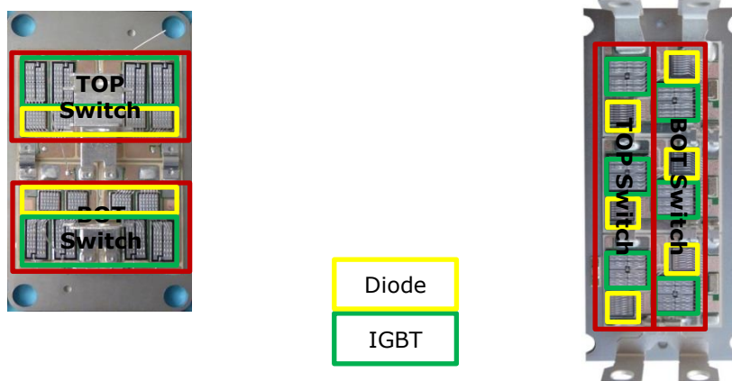
Figure 7: Thermal resistances R_{th(c-s)} of 450A-SEMITRANS 3 (left) and 450A-SEMiX 3s (right) for different situations of thermal coupling between switches accordingly Table 4
