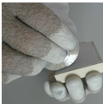
Figure 21: Using a roller gauge to measure the thickness of paste on a MiniSKiiP module
