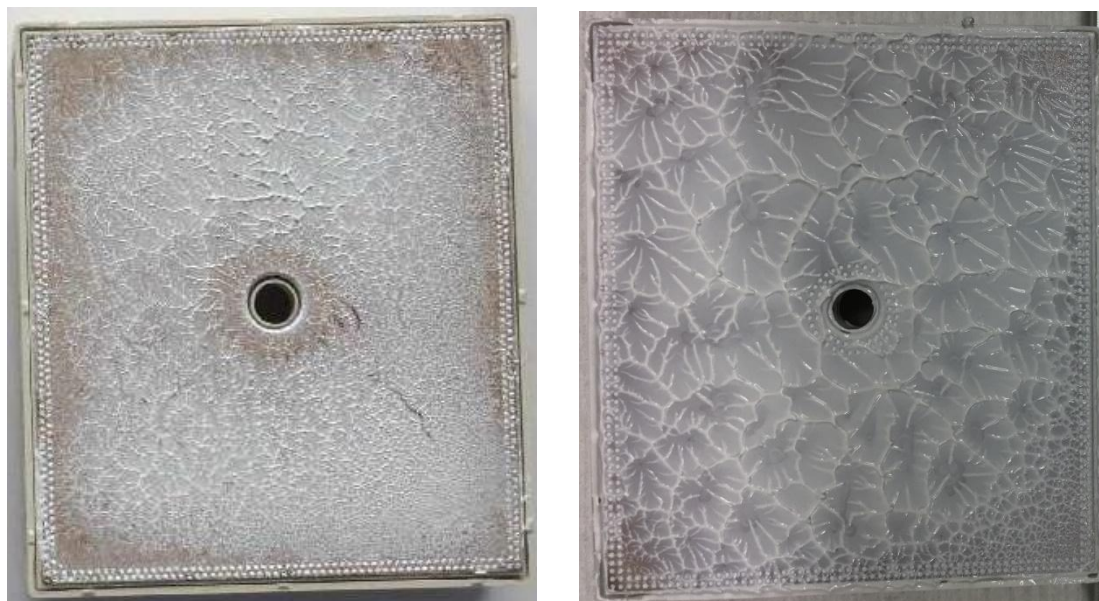
Figure 25: Correct distribution of paste (L) and too much paste (R) on module underside
