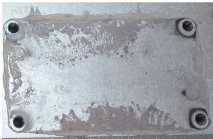
Figure 27: Mounting position of SEMITRANS module showing signs of pump-out after repeated thermal cycling
