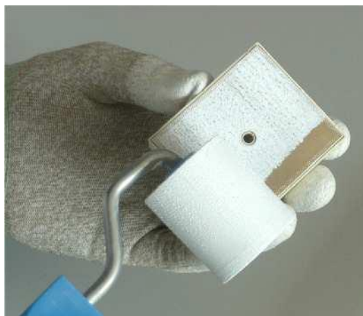
Figure 7: Applying paste to a MiniSKiiP module
