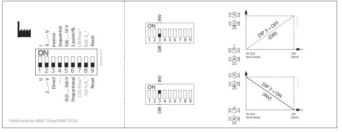
The actuator has a selection of DIP switches under the removable cover. The switch provides the following functions:
