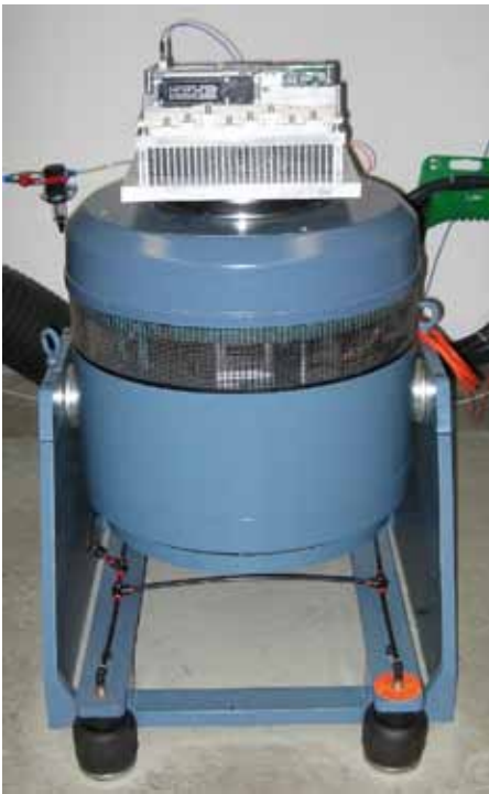
Figure 2.7.4 SKiiP system on a vibrating plate
