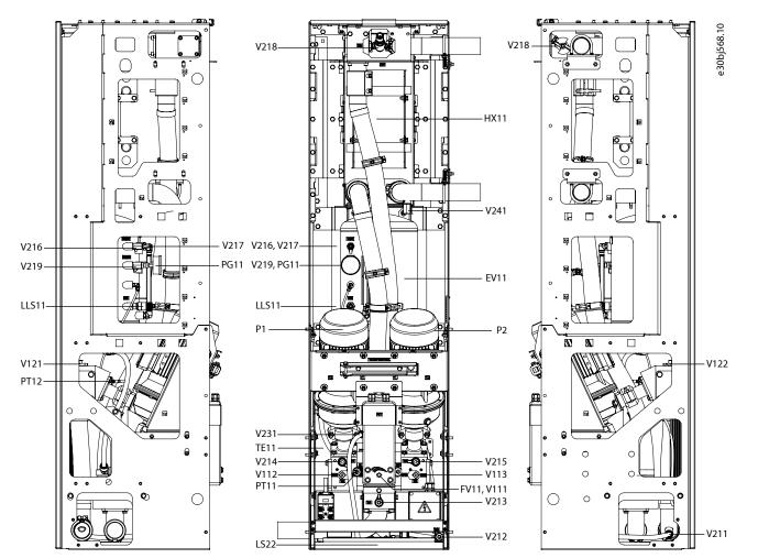
Figure 19: Location of Valves and Instrumentation in Dual-pump 76 kW and 152 kW Cooling Module
