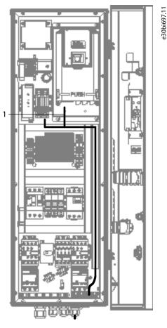
Figure 30: Control Compartment Wiring Route
