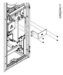
Figure 20: Removing the Mounting Plate of the Valve Actuator
