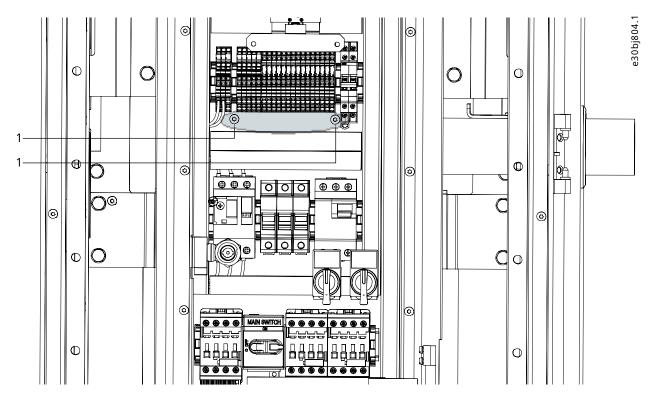
Figure 5: Transportation Screws of the Control Compartment
