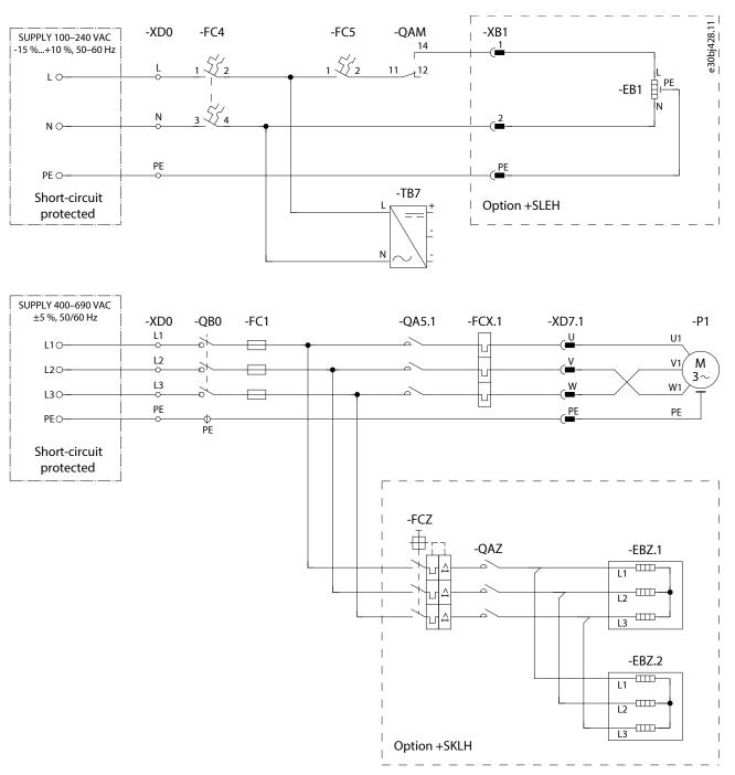
Figure 52: Wiring Diagram for Single-pump Cooling Module with External Auxiliary Supply
