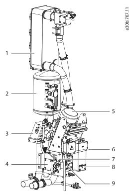
Figure 12: Components of the Drive Circuit
