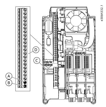
Figure 34: Ethernet and RS485 Connections in the Control Unit
