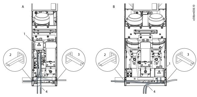
Figure 27: Installing the Mains Cables
