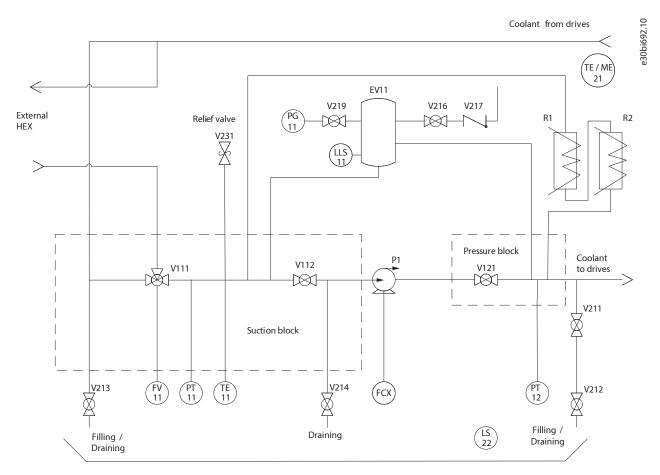
Figure 47: Piping and Instrumentation Diagram of the Single-pump Cooling Module with an External Heat Exchanger
