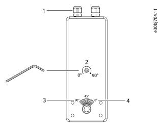
Figure 24: Installation and Manual Adjustment of the 3-way Valve Actuator
