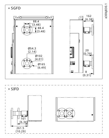
Figure 41: Dimensions of the Optional DIN Flanges, +SGFD and +SIFD, in mm (in)
