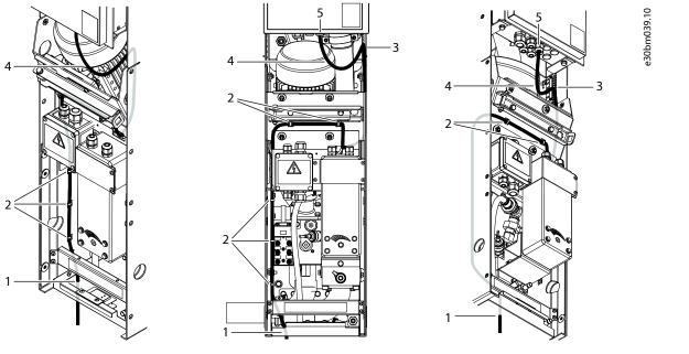
Figure 28: Control Cable Routing of the Cooling Module with 1 Pump
