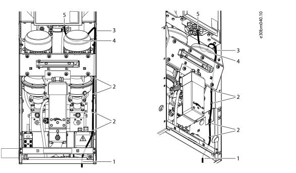
Figure 29: Control Cable Routing of the Cooling Module with 2 Pumps
