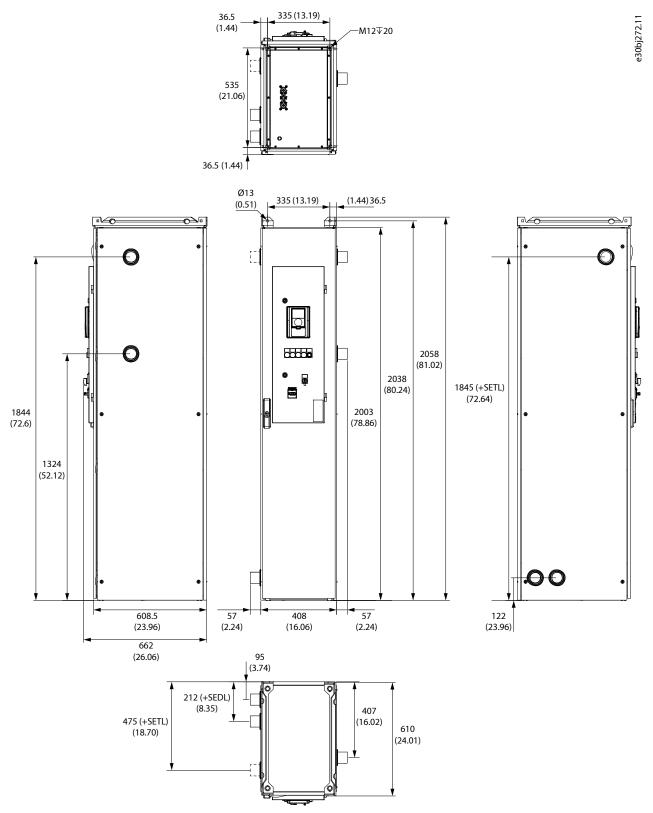
Figure 37: Dimensions of the Single-pump Enclosed Cooling Module in mm (in), Drive Circuit Pipes on the Left
