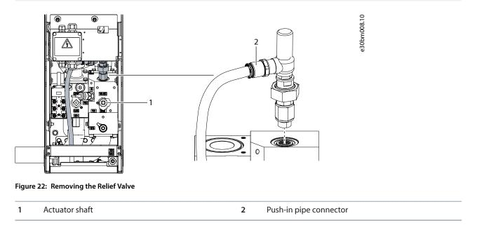
5. Place a plug into the threaded hole. The plug is included in the accessories bag.
