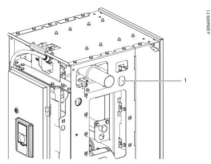
Figure 3: Vertical Lifting of the Standalone Cooling Module
