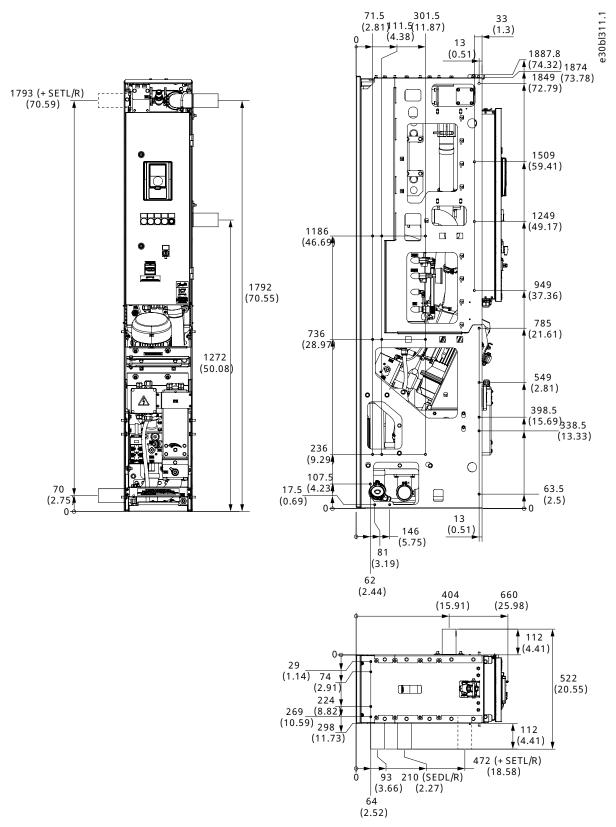
Figure 35: Dimensions of the Single-pump Standalone Cooling Module in mm (in)
