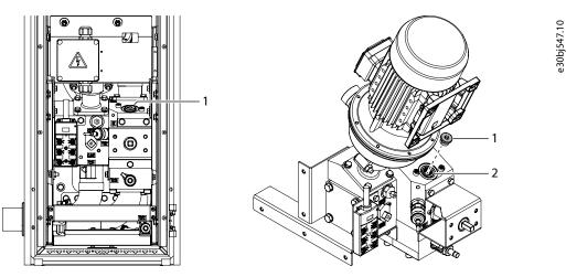
Figure 23: Plugging the Hole of the Relief Valve
