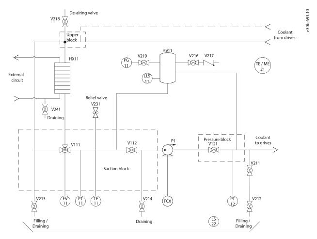
Figure 48: Piping and Instrumentation Diagram of the Single-pump 76 kW and 152 kW Cooling Module
