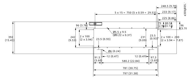
Figure 6: Dimensions for the Cut-out on the Cabinet Door in mm, Single-pump Cabinet
