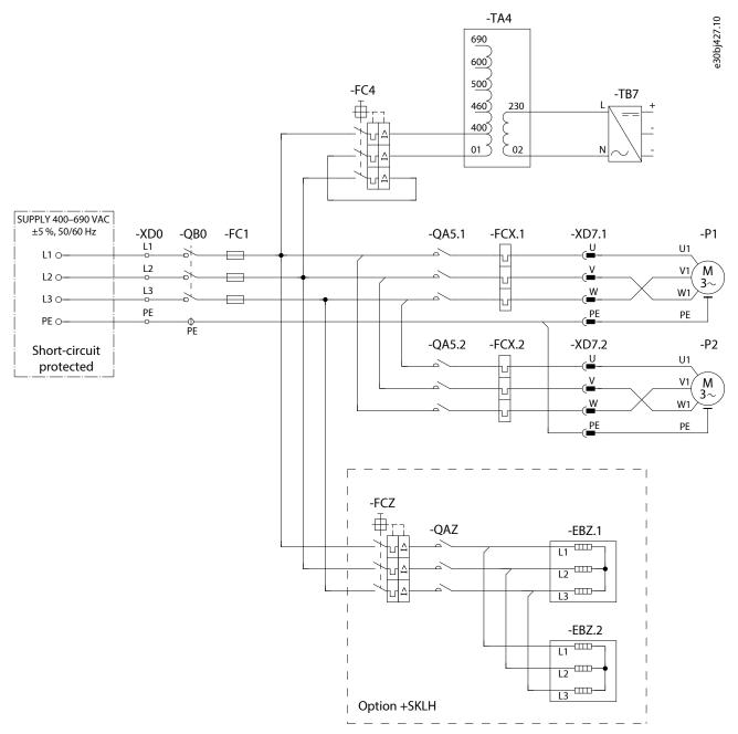
Figure 54: Wiring Diagram for Dual-pump Cooling Module with Auxiliary Transformer
