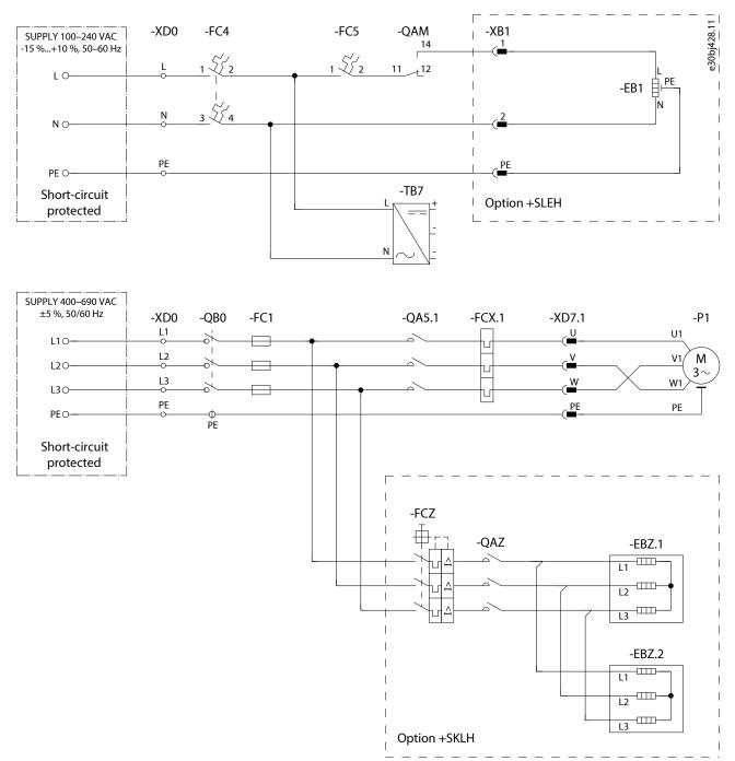
Figure 55: Wiring Diagram for Single-pump Cooling Module with External Auxiliary Supply
