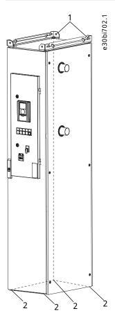
Figure 10: Mounting Holes of the Enclosed Cooling Module
