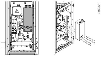
Figure 21: Removing the Valve Actuator
