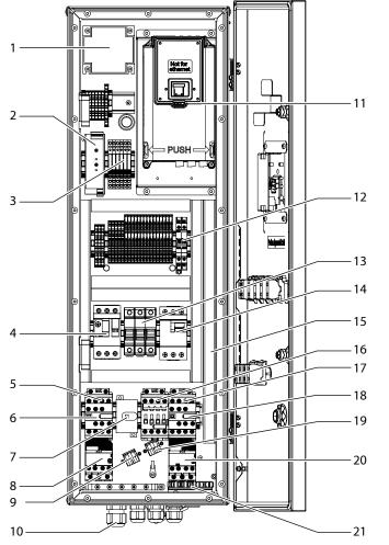
Figure 32: Control Compartment, Door Open
