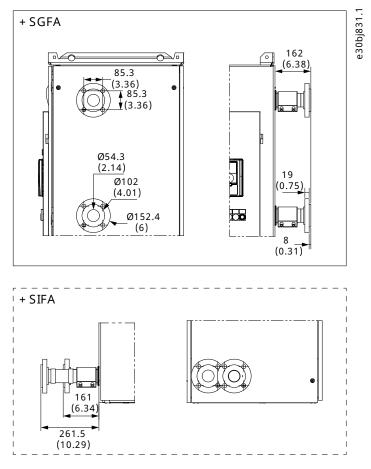
Figure 42: Dimensions of the Optional ANSI Flanges, +SGFA and +SIFA, in mm (in)
