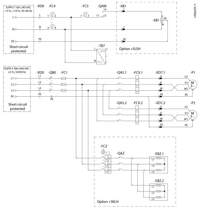
Figure 53: Wiring Diagram for Dual-pump Cooling Module with External Auxiliary Supply
