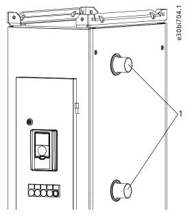
Figure 15: Pipe Connections at the Top
