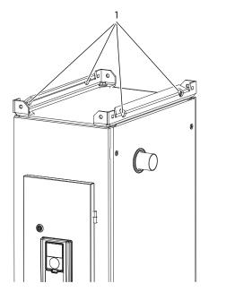
Figure 2: Lifting the Enclosed Cooling Module
