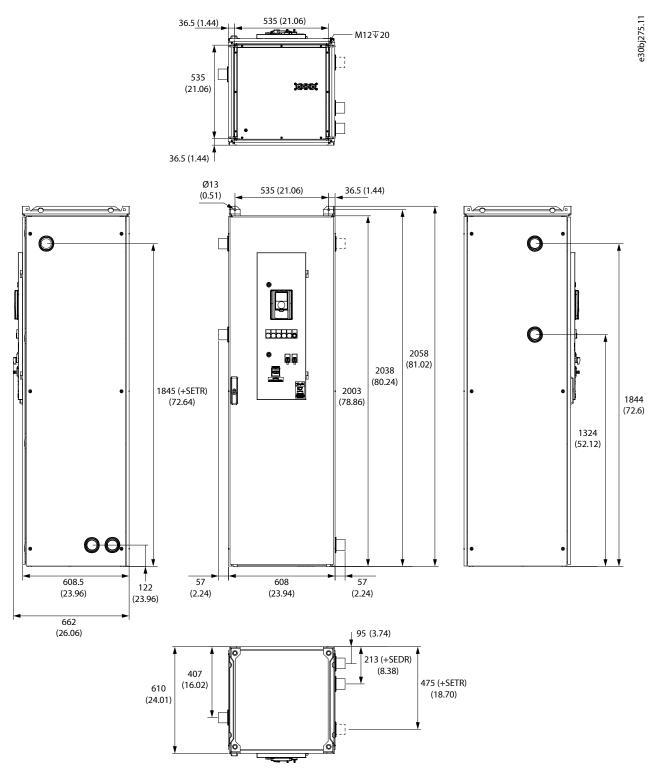
Figure 40: Dimensions of the Dual-pump Enclosed Cooling Module in mm (in), Drive Circuit Pipes on the Right
