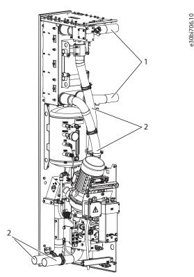
Figure 11: Circulation of Liquid in the 2 Circuits of the Cooling Module
