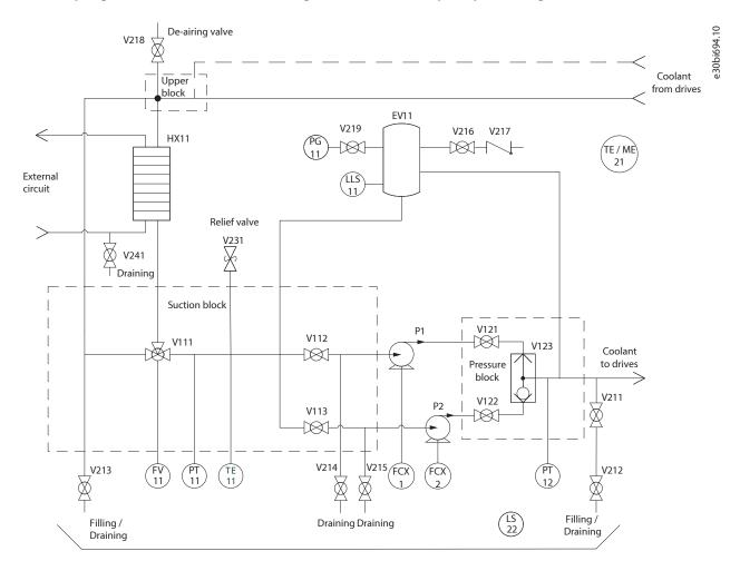
Figure 49: Piping and Instrumentation Diagram of the Dual-pump 76 kW and 152 kW Cooling Module
