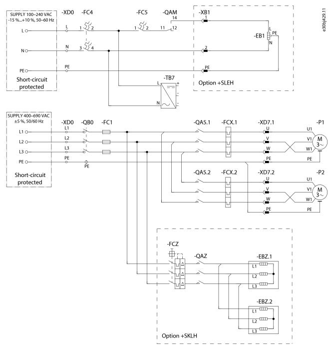
Figure 56: Wiring Diagram for Dual-pump Cooling Module with External Auxiliary Supply
