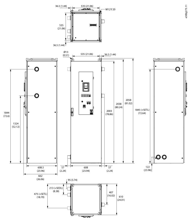
Figure 38: Dimensions of the Dual-pump Enclosed Cooling Module in mm (in), Drive Circuit Pipes on the Left
