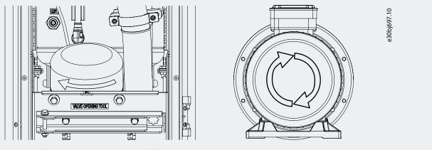
Figure 26: The Correct Rotation Direction of the Pump Motor
