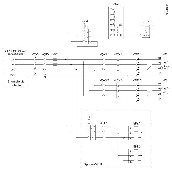
Figure 51: Wiring Diagram for Dual-pump Cooling Module with Auxiliary Transformer
