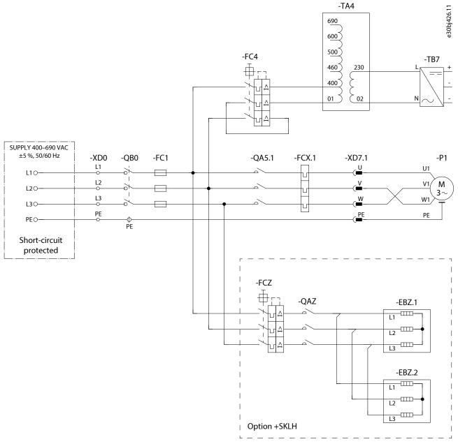
Figure 50: Wiring Diagram for Single-pump Cooling Module with Auxiliary Transformer
