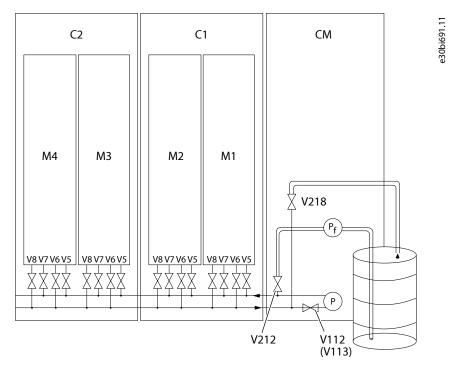
Figure 25: Filling the Cooling System
