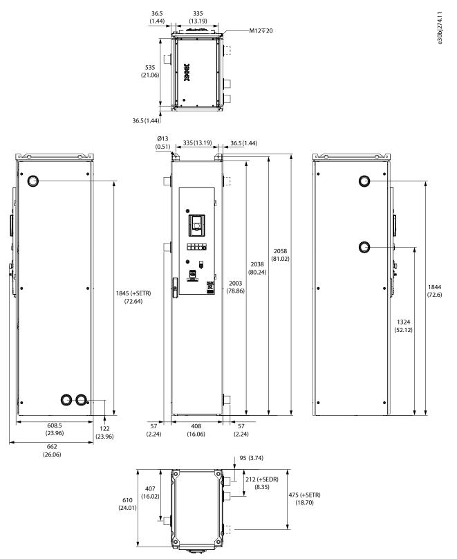
Figure 39: Dimensions of the Single-pump Enclosed Cooling Module in mm (in), Drive Circuit Pipes on the Right
