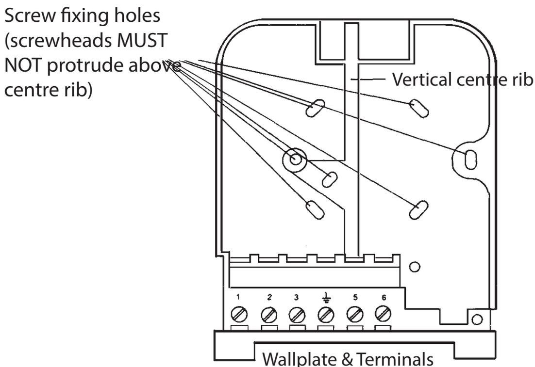
4. Surface cables can only enter from below the unit. Cut an appropriate cable aperture in the wiring cover. If the wallplate is mounted on a plaster box, cables can enter from the rear below the terminal block.
