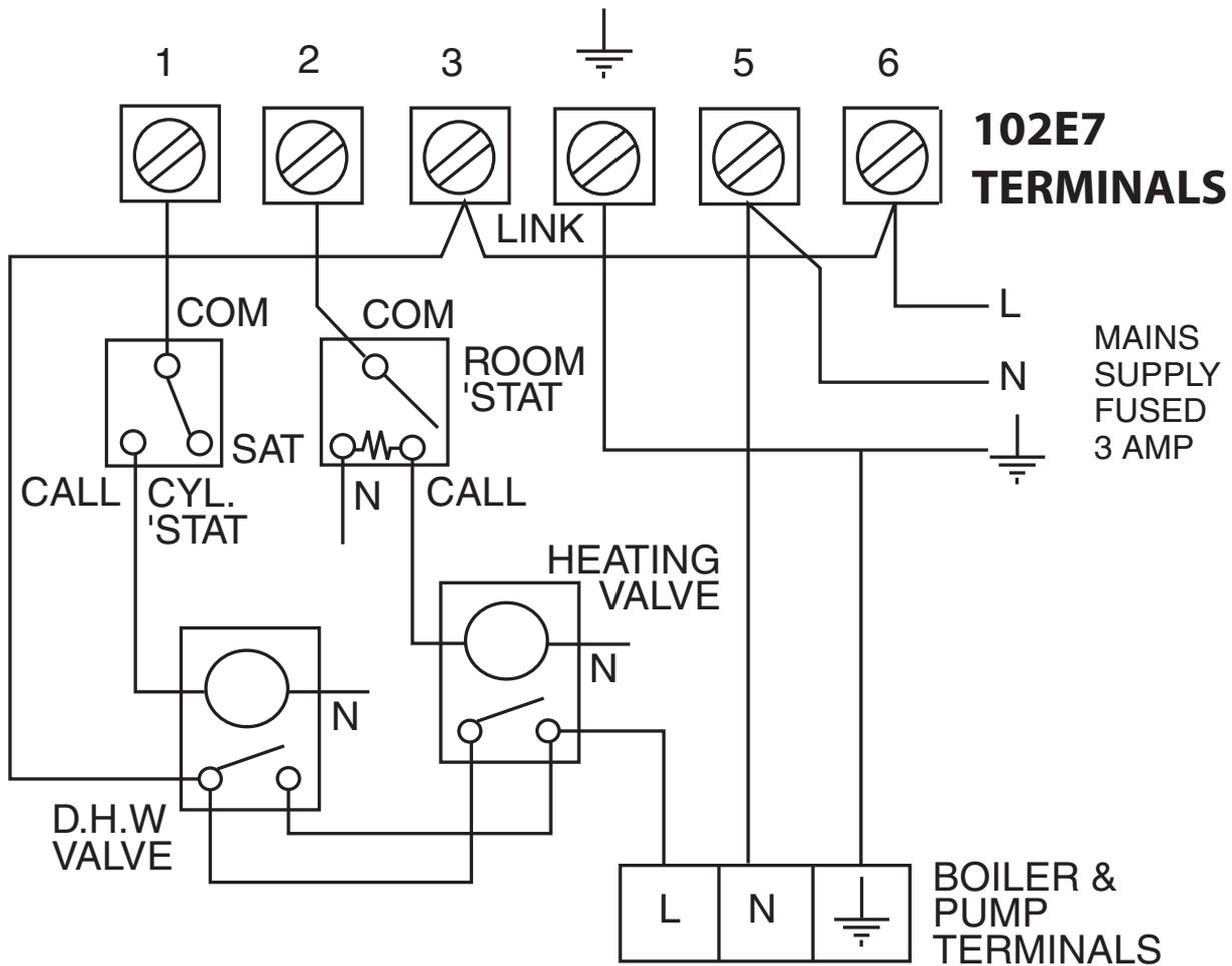
The above control system is available as the Danfoss Randall 102E7 HEATPLAN pack, which also includes the RMT room thermostat, AT cylinder thermostat, two 22mm HPP zone valves and a WB12 wiring box.
