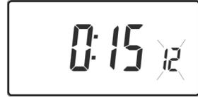
The optimum start control must be adjusted to match the building energy characteristics. Use the **Λ** and **V** keys to selected the required pre-heat period. The table below suggests typical settings.
