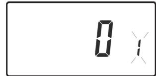
Use **Λ** and **V** keys to enable or disable the function (1=enabled, 0=disabled).
