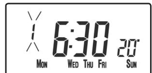
b) Use the + and - buttons to adjust the **TIME** (press and hold to change in 10 minute increments).
