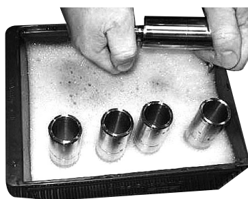
16. Note: If pistons are replaced, place new pistons in clean filtered water for a couple of minutes. Exercise piston shoes to make them "run" smoother.
