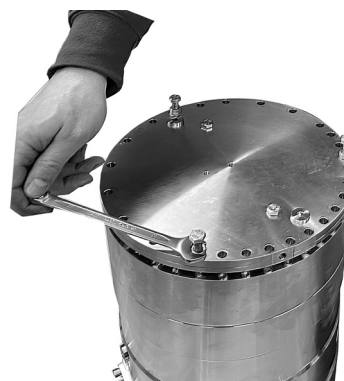
19. Lubricate the O-ring on the end flange. Align the pinhole in the flange with the pin in the housing. Install the three bolts and nuts from the tool kit. Turn each nut one round at a time to ensure mounting flange is mounted as straight downwards as possible. Be careful not to squeeze the O-ring.
