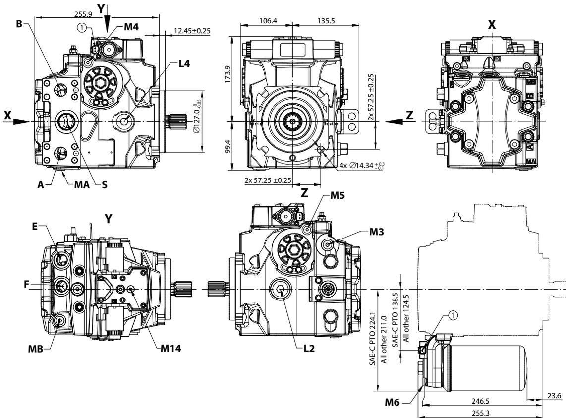
**A/B** system ports: Ø25.4–450 bar; Split flange boss per ISO 6162
