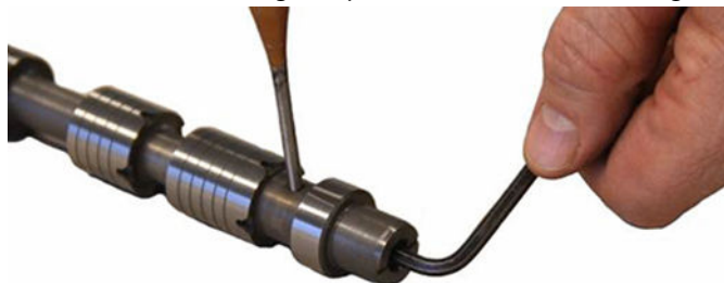
Dismantled directional spool (25) and orifice (26)
