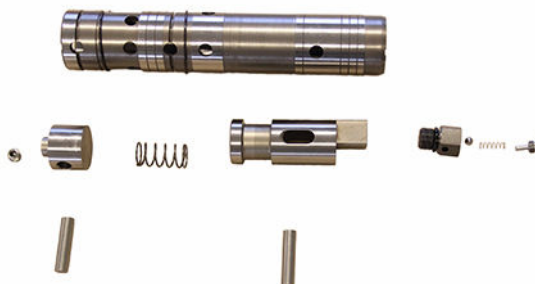
Dismantled amplifier spool
