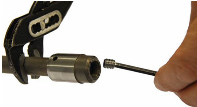
Dismantled priority valve spool (25) with throttle/check valve (4) and orifice, dynamic (11)
