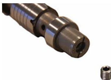
Dismantled directional spool (25) and orifice (26)
