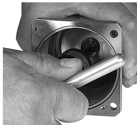
17. Tighten to a torque of 10 \pm 1 Nm.
