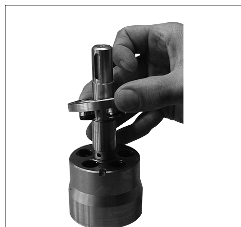
14. Remove the valve plate.
