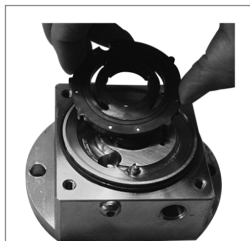
16. Remove the port plate from the flange.
