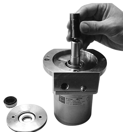
25. Fit the hollow bush onto the shaft.
