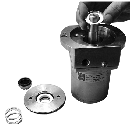
23. Mount the washer with the edge pointing upwards.
