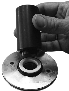
22. Wet the shaft seal with water and mount it in the front cover. Ensure that it is pressed to the bottom.
