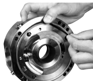
4. Mount O-ring in port plate.
