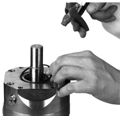
33. Spray with water and mount O-ring.
