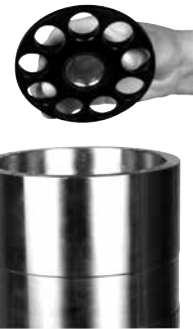
20. Place retainer plate on top of retainer ball.
