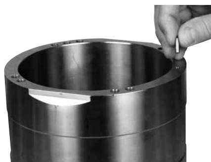
3. Mount 1 guide pin in housing.
