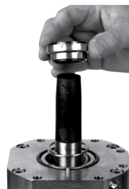
40. Mount sealing (smallest diameter pointing down).
