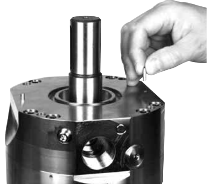
32. Turn pump upside down and mount 2 guide pins.
