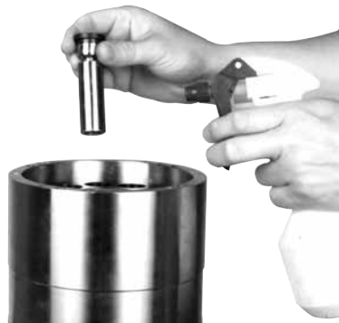
21. Spray with water and mount pistons.
