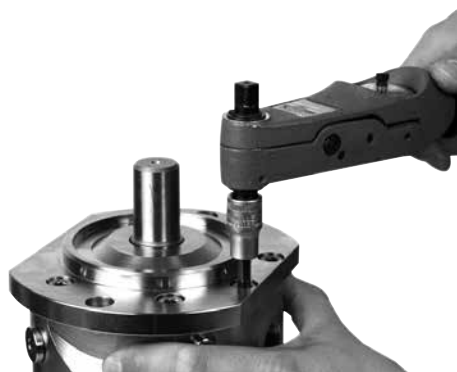
43. Tighten screws to 30Nm.
