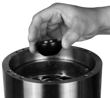
13. Remove retainer ball.
