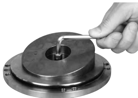
28. Loosen and remove screw from swash plate.
