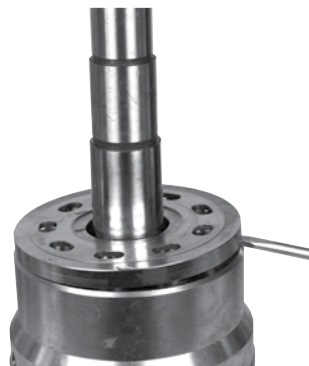
23. Loosen thrust plate from cylinder barrel.
