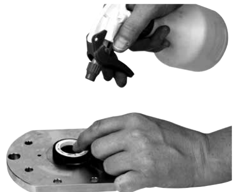
34. Spray shaft sealing with water before mounting.
