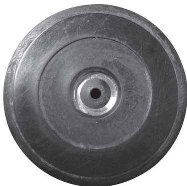
1. Picture 1: No wear or cavitation of the piston shoe. New inspection is required in 4,000 hours.
