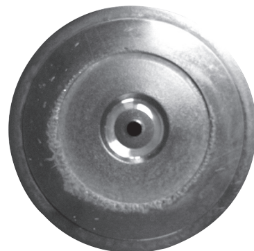
2. Picture 2: Cavitation of the piston shoes. New inspection is required in 2,000 hours.
