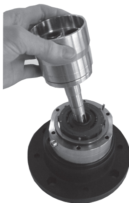
7. Remove the cylinder barrel.
