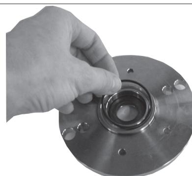
16. Hold the pump together and carefully turn it over to rest on the housing. To prevent seizing-up, lubricate the threads on the 2 screws and screw them into the port flange and the housing. Use Molykote D paste from Dow Corning or Klüber UH1 84-201 from Klüber lubrication. Tighten the 2 flange screws according to exploded view.
