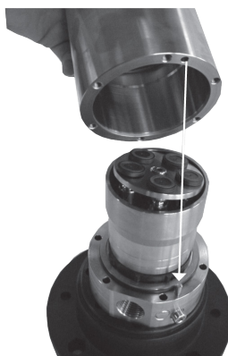
15. Position the housing on the port flange and over the guide pin.
