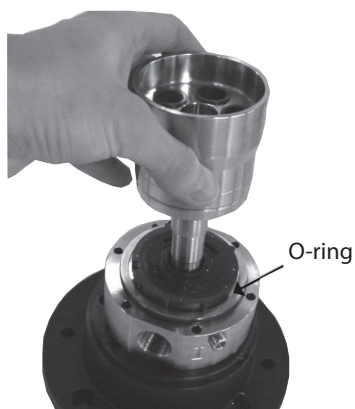
13. Replace O-ring on the port flange and position the new cylinder barrel on the port plate.
