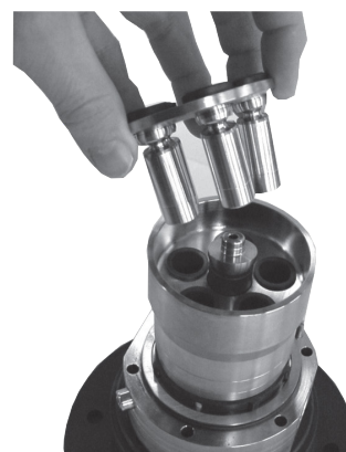
14. Position the new spring, new spring guide, new retaining ball, new retainer and new pistons.
