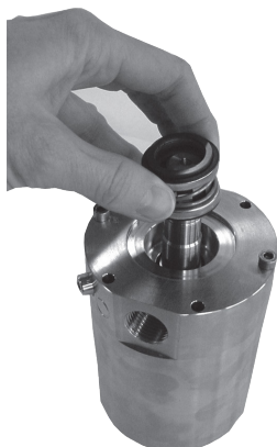
17. Mount the new shaft seal following the instructions on page
