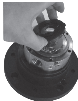
8. Remove the port plate and guide pin.
