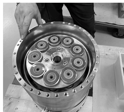
17. Place pistons in retainer plate and cylinder barrel. When pistons are placed, tilt retainer plate for easier placement of swash plate. If swash plate has been disassembled from mounting flange, see page 7 for assembly of swash plate.
