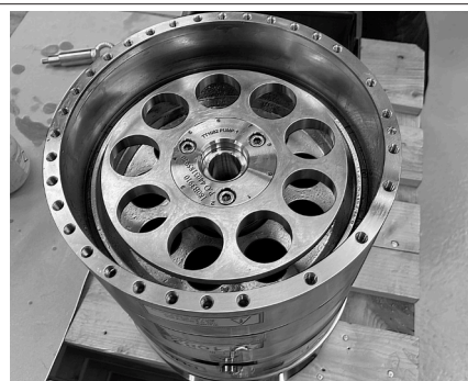
15. Lubricate the cylinder barrel with clean filtered water. Install the Retainer guide in the cylinder barrel and place the complete retainer plate with the ball towards the bearing. Retainer ball and retainer plate in the cylinder barrel.
